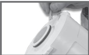
Remove cartridge and inspect O-ring. Replace if damaged. Reinsert cartridge and verify that it is installed correctly. When viewed from above, white locking tabs on cartridge should be visible in four openings on filter head.
